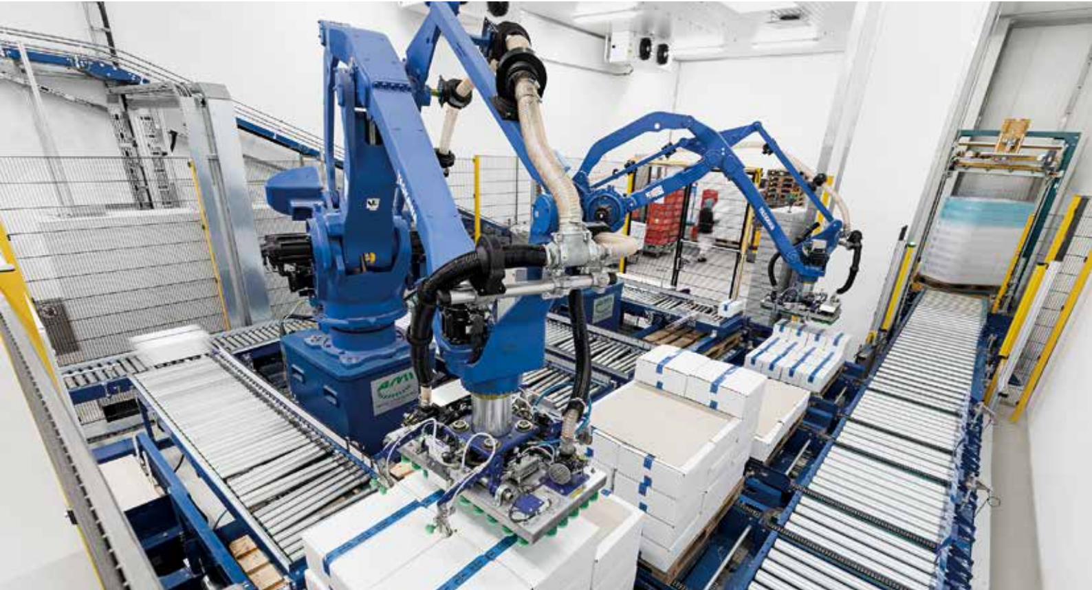
Palletiser with layer pad inserter
