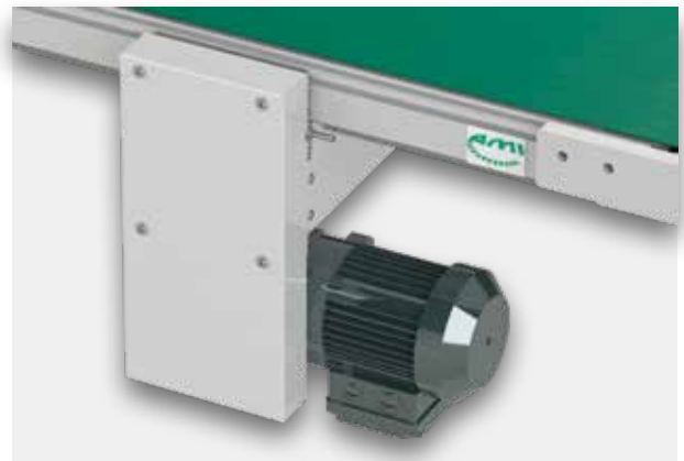
Centre drive with intermediate gear unit
