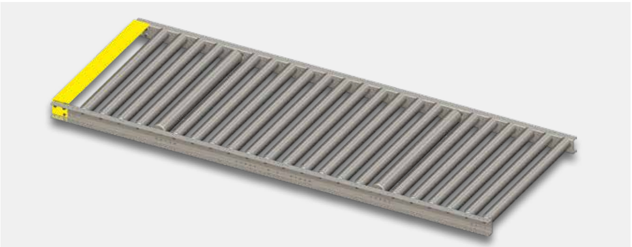
Manual pallet-loading station PAS 60-0 with full-length rollers
