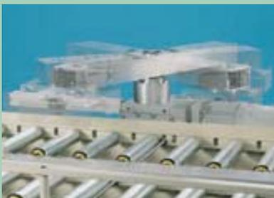
The AMI rotary extractor is at the heart of modern consignment and sorting equipment. Plastic bins, cardboard boxes or single packages are precisely and safely extracted from the conveyor on either parallel or cross belts. Take advantage of the flexibility of the AMI rotary extractor: It is installed in the position where it is needed at the conveyor and can be easily relocated in the event of modernization, reconstruction or logis-
